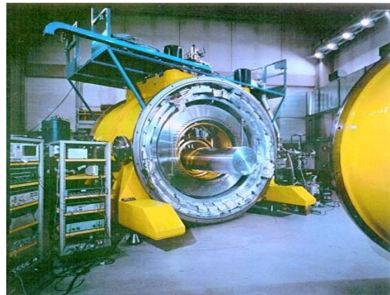
Figure 17: The antenna NAUTILUS at Frascati, showing the bar and its cryogenic shields. (Source https://malagabay.wordpress.com/2015/07/23/the-syncopated-sidereal-shake )
